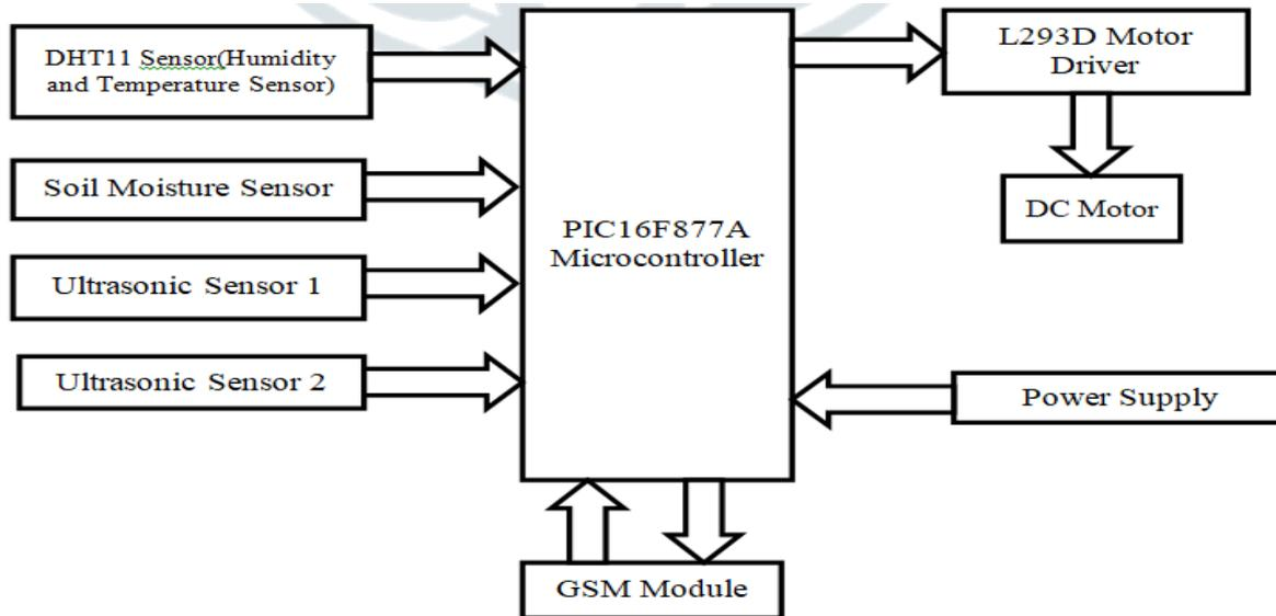
Figure 1: Real time monitoring System
